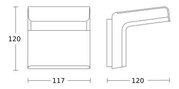
Possible mounting height: 1,80 m - 2,00 m Orange: radial and tangential 3 scalable axes
